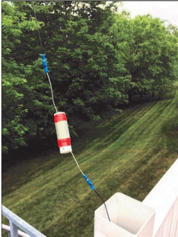
36 Turn 40 Meter Coil and adding and trimming a second 30' horizontal Radial element
